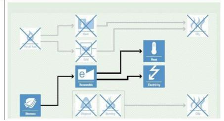
The proposed project activity uses bagasse as fuel for cogeneration unit. The bagasse being a renewable bio- mass fuel does not add any net carbon-dioxide to the atmosphere because of the carbon recycling during growth of sugar cane. Therefore, the project activity will lead to zero CO2 on-site emissions associated with bagasse combustion.
